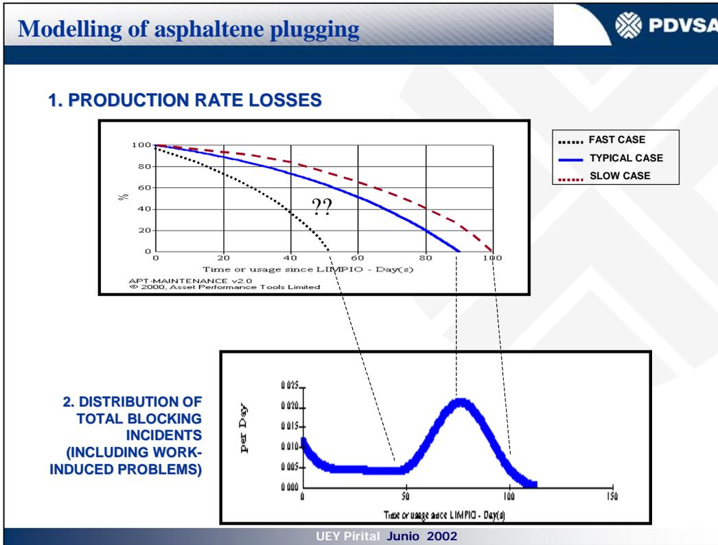
Figure 5. Deterioration modelling and reliability pattern description
